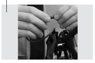
Connect the EPS cable with the front derailleur.
